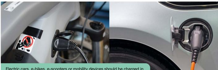
Electric cars, e-bikes, e-scooters or mobility devices should be charged in a garage, shed or carport away from living spaces and flammable materials. **DO NOT** charge or store batteries in exit paths.
